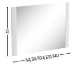
Mirror with side trim to match the furniture. Lighting LED IP44 class II - 4.8 w/ml - 350 lm/ml -  $6000 ^{\circ} \text{K}$
