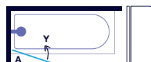
A - Moving Panel Y - Radius of swing= 733mm Door swings 90° inwards and outwards
